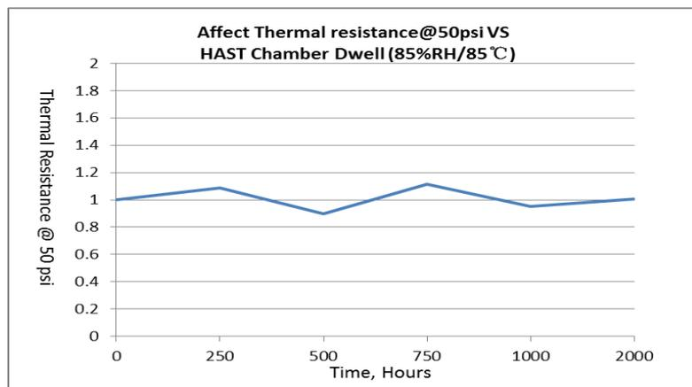
Graph1, 2, 3 show the results of HAST chamber aging effect, the dielectric properties of Tgard300 were not affected by the exposure to 85 % relative humidity and 85 °C of 2000 hours, and the thermal resistance at 10psi was stable with time increase, and it was fluctuated slightly within 10% range at 50 psi and then eventually stabilizes as time of exposure increases.
