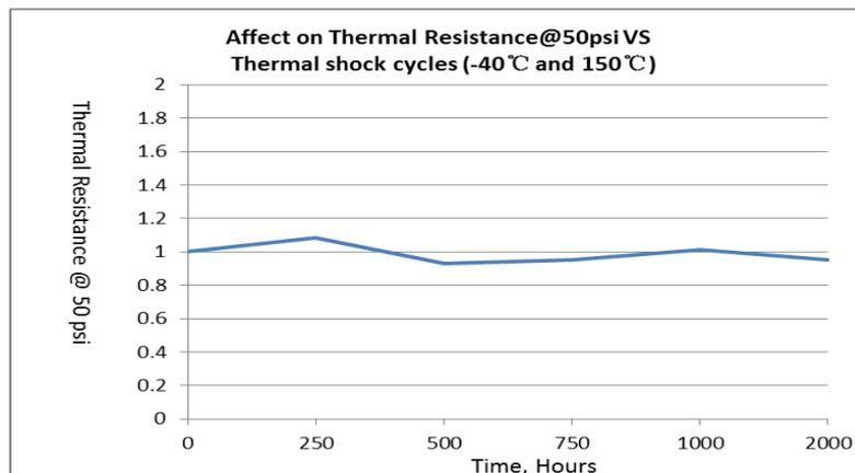
Graph7, 8, 9 indicate that Tgard300 maintains its thermal, and dielectric qualities after exposure to 2000 thermal shock cycles between -40 °C and + 150 °C.
