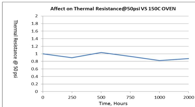
Graph4, 5, 6 show the results that dielectric properties and thermal resistance at 10psi were stable during the testing, and it was fluctuated slightly at 50 psi as time of exposure increases.
