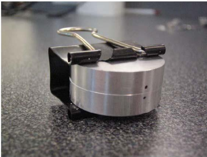
Picture #2 Aluminum disks clamped with PCM between them
