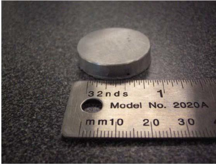
Appendix Picture #1 Aluminum disk used for reliability testing
