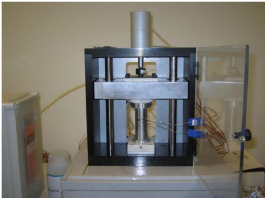
Picture #4 ASTM D5470 thermal resistance tester
