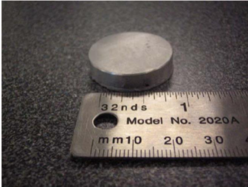
Picture #1 Aluminum disk used for reliability testing
